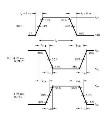
Figure 6. AC Waveforms
