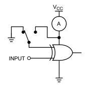
Input = AC Waveform; PRR = Variable; Duty Cycle = 50%.
