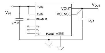
Figure 6: Application Circuit, EP5358HUI,.
