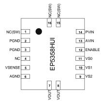
Figure 4: EP5358HUI Pin Out Diagram (Top View)
