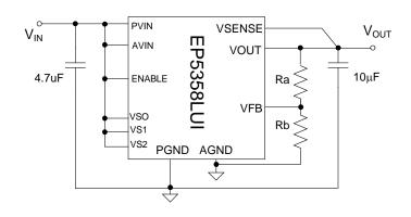
Figure 8: EP5358LUI using external divider
