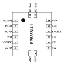
Figure 3: EP5358LUI Pin Out Diagram (Top View)
