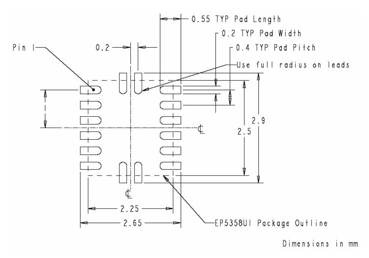
Figure 11: EP5358xUI Package PCB Footprint
