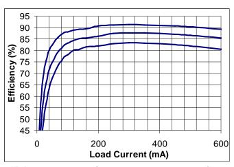
Efficiency vs. Load Current:  $V_{IN} = 3.7V$ ,  $V_{OUT}$  (from top to bottom) = 2.5, 1.8, 1.2V
