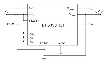
Figure 2: Typical Application Schematic
