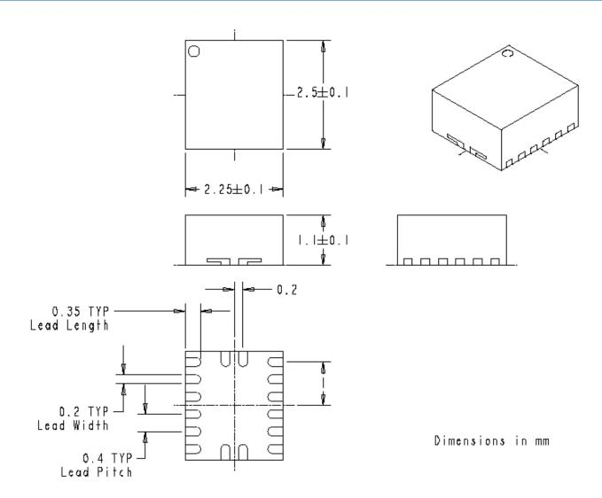
Figure 12: EN5358xUI Package Dimensions
