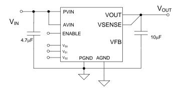
Figure 7: Application Circuit, EP5358LUI, showing the  $V_{\text{FB}}$  function.
