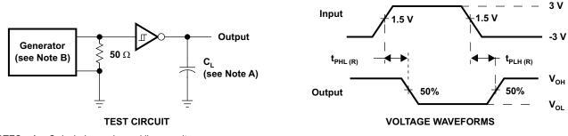
NOTES: A. C<sub>L</sub> includes probe and jig capacitance. B. The pulse generator has the following characteristics:  $Z_0 = 50 \ \Omega$ , 50% duty cycle,  $t_r \le 10 \text{ ns}$ ,  $t_f \le 10 \text{ ns}$ .
