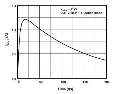
Figure 6. Typical HBM Current Waveform
