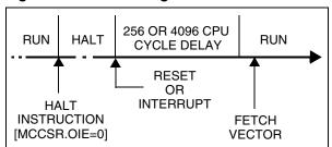
Figure 26. HALT Mode Flow-chart
