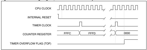
Note: The MCU is in reset state when the internal reset signal is high, when it is low the MCU is running.
