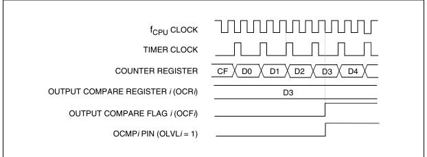
Figure 67. Output Compare Timing Diagram,  $f_{TIMER} = f_{CPU}/4$
