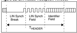
The time-out counter is enabled at each break detection. It is stopped in the following conditions:
