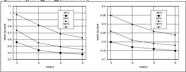
Figure 110. Typical  $V_{OL}$  vs  $V_{DD}$  (High-sink I/Os)
