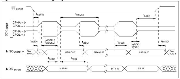
Figure 118. SPI Master Timing Diagram<sup>1)</sup>
