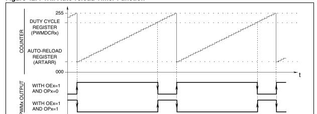
Figure 42. PWM Auto-reload Timer Function
