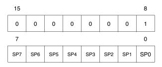
The Stack Pointer is a 16-bit register which is always pointing to the next free location in the stack. It is then decremented after data has been pushed onto the stack and incremented before data is popped from the stack (see Figure 2).
