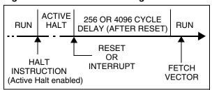
Figure 28. ACTIVE HALT Mode Flow-chart
