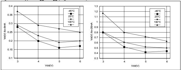
Figure 111. Typical  $V_{OH}$  vs  $V_{DD}$
