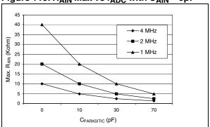
Figure 120. Recommended C<sub>AIN</sub>/R<sub>AIN</sub> Values<sup>3)</sup>
