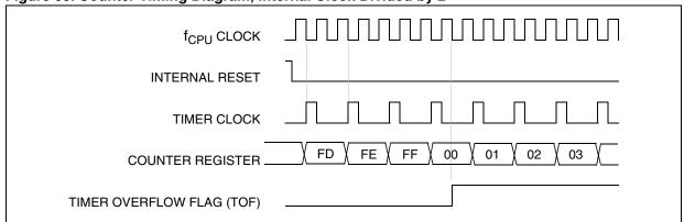
Figure 61. Counter Timing Diagram, Internal Clock Divided by 4
