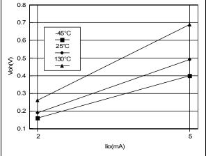
Figure 107. Typical V<sub>OL</sub> at V<sub>DD</sub> = 5V (High-sink)
