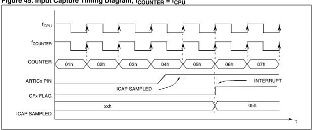
Figure 45. Input Capture Timing Diagram, f<sub>COUNTER</sub> = f<sub>CPU</sub>
