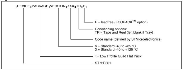
Figure 131. FASTROM Factory Coded Device Types
