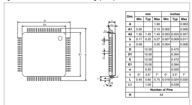
Figure 126. 64-Pin Low Profile Quad Flat Package (10 x10)
