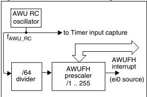
As soon as HALT mode is entered, and if the AWUEN bit has been set in the AWUCSR register, the AWU RC oscillator provides a clock signal (f<sub>AWU\_RC</sub>). Its frequency is divided by a fixed divider and a programmable prescaler controlled by the AWUPR register. The output of this prescaler provides the delay time. When the delay has elapsed the AWUF flag is set by hardware and an interrupt wakes up the MCU from Halt mode. At the same time the main oscillator is immediately turned on
