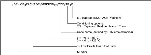
Figure 129. ROM Factory Coded Device Types
