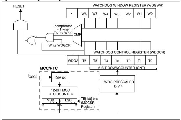
The application program must write in the WDGCR register at regular intervals during normal operation to prevent an MCU reset. This operation must occur only when the counter value is lower than the window register value. The value to be stored in the WDGCR register must be between FFh and C0h (see Figure 2):
