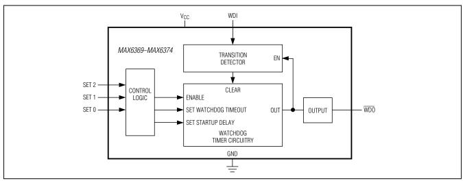
Figure 1. Functional Diagram
