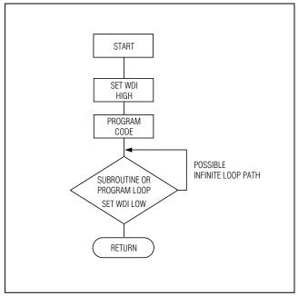
Figure 4. Watchdog Flow Diagram
