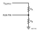
Figure 2. Undervoltage Lockout Resistive Divider
