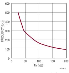
Figure 1. Timing Resistor  $(R_T)$  Value
