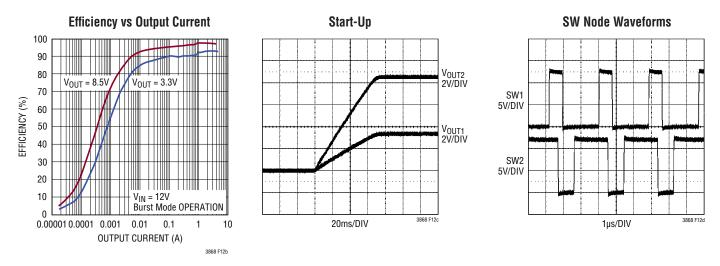
Figure 12. High Efficiency Dual 8.5V/3.3V Step-Down Converter
