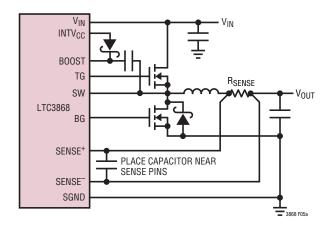
(5a) Using a Resistor to Sense Current
