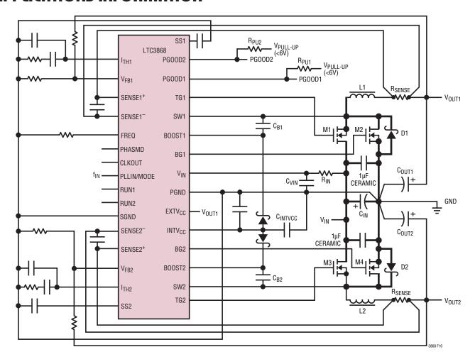
Figure 10. Recommended Printed Circuit Layout Diagram
