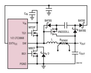
Figure 8. Capacitive Charge Pump for EXTV<sub>CC</sub>
