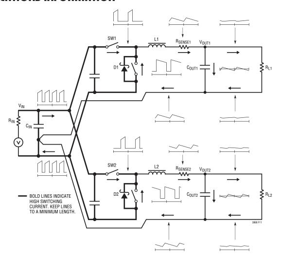
Figure 11. Branch Current Waveforms
