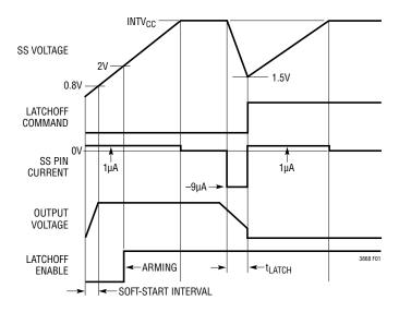
Figure 1. Latchoff Timing Diagram
