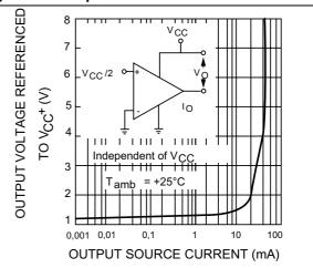
Figure 9. Output characteristics
