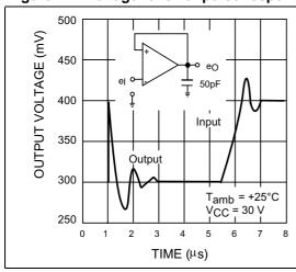
Figure 12. Input voltage range
