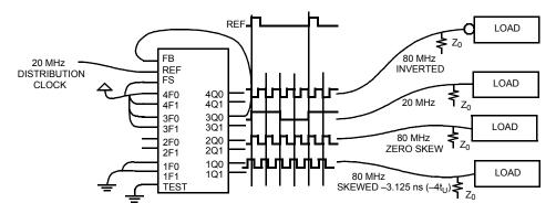
Figure 9. Board-to-Board Clock Distribution
