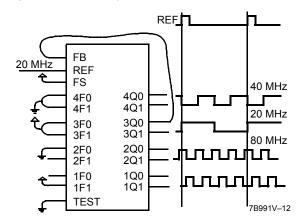
Figure 6 shows the LVPSCB configured as a clock multiplier. The 3Q0 output is programmed to divide by four and is sent back to FB. This causes the PLL to increase its frequency until the 3Q0 and 3Q1 outputs are locked at 20 MHz, while the 1Qx and 2Qx outputs run at 80 MHz. The 4Q0 and 4Q1 outputs are programmed to divide by two that results in a 40 MHz waveform at these outputs. Note that the 20 and 40 MHz clocks fall simultaneously and are out of phase on their rising edge. This enables
