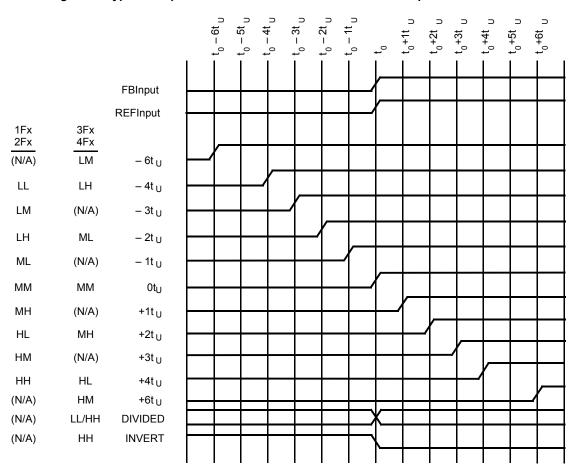
Figure 2. Typical Outputs with Fb Connected to a Zero Skew Output Test Mode<sup>[4]</sup>
