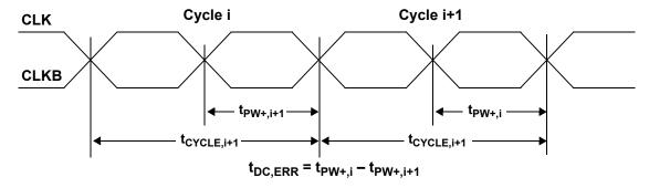
Figure 11. Cycle-to-cycle Duty Cycle Error
