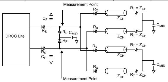
Figure 4. Output Driving Two Channels
