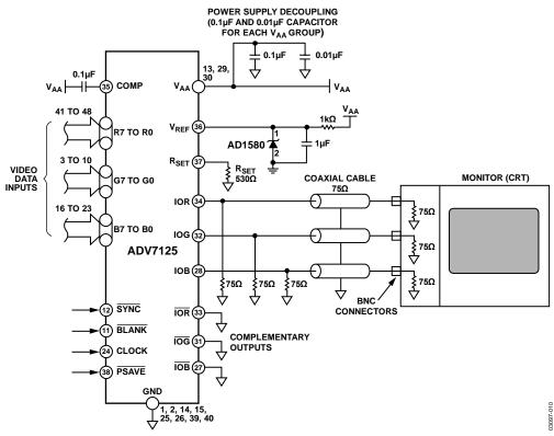
Figure 12. Typical Connection Diagram
