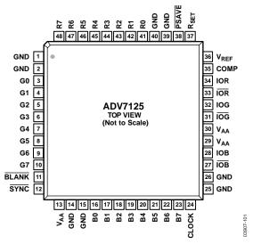
Figure 5. LQFP Pin Configuration
