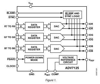
The ADV7125 is fabricated in a 5 V CMOS process. Its monolithic CMOS construction ensures greater functionality with lower power dissipation. The ADV7125 is available in 48-lead LQFP and 48-lead LFCSP packages.
