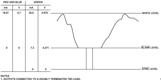
2.  $V_{REF}$  = 1.235V,  $R_{SET}$  = 530Ω. 3. RS-343 LEVELS AND TOLERANCES ASSUMED ON ALL LEVELS.
