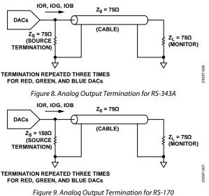
More detailed information regarding load terminations for various output configurations, including RS-343A and RS-170, is available in the AN-205 Application Note, *Video Formats and Required Load Terminations*.
