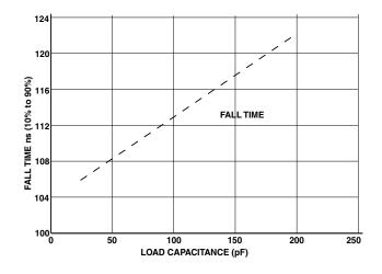
Figure 52. Typical Fall Time (10% to 90%) vs. Load Capacitance for Driver E at V<sub>DDEXT</sub> = 3.65 V (MAX)
