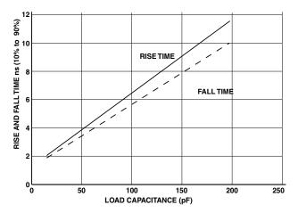
Figure 44. Typical Rise and Fall Times (10% to 90%) vs. Load Capacitance for Driver A at V<sub>DDEXT</sub> = 3.65 V (MAX)
