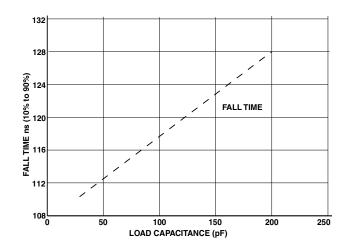
Figure 51. Typical Fall Time (10% to 90%) vs. Load Capacitance for Driver E at  $V_{DDEXT} = 2.7 V$  (MIN)
