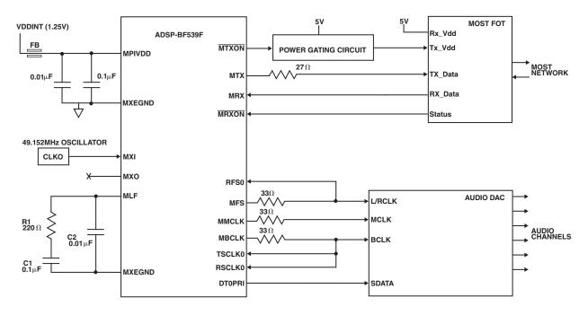
Figure 9. Example Connections of ADSP-BF539/ADSP-BF539F to MOST Network
