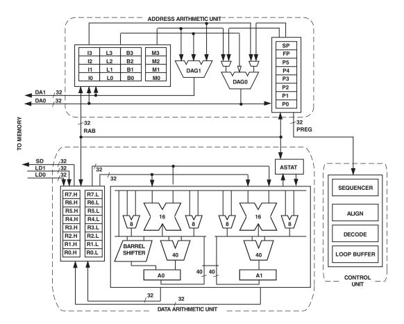
Figure 2. Blackfin Processor Core
