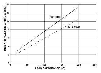
Figure 43. Typical Rise and Fall Times (10% to 90%) vs. Load Capacitance for Driver A at V<sub>DDEXT</sub> = 2.7 V (MIN)
