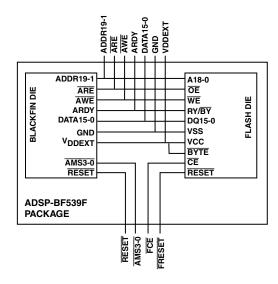
Figure 4. Internal Connection of Flash Memory (ADSP-BF539Fx)
