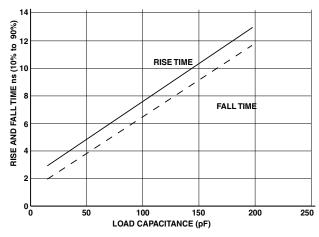
Figure 50. Typical Rise and Fall Times (10% to 90%) vs. Load Capacitance for Driver D at  $V_{DDEXT} = 3.65 V (MAX)$
