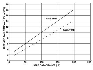
Figure 48. Typical Rise and Fall Times (10% to 90%) vs. Load Capacitance for Driver C at V<sub>DDEXT</sub> = 3.65 V (MAX)
