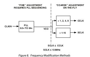
All on-chip peripherals are clocked by the system clock (SCLK). The system clock frequency is programmable by means of the SSEL3–0 bits of the PLL\_DIV register. The values programmed into the SSEL fields define a divide ratio between the PLL output (VCO) and the system clock. SCLK divider values are 1 through 15. Table 7 illustrates typical system clock ratios.
