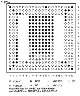
Figure 53. 316-Ball CSP\_BGA Ball Assignment (Top View)
