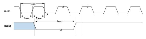
Figure 11. Clock and Reset Timing
