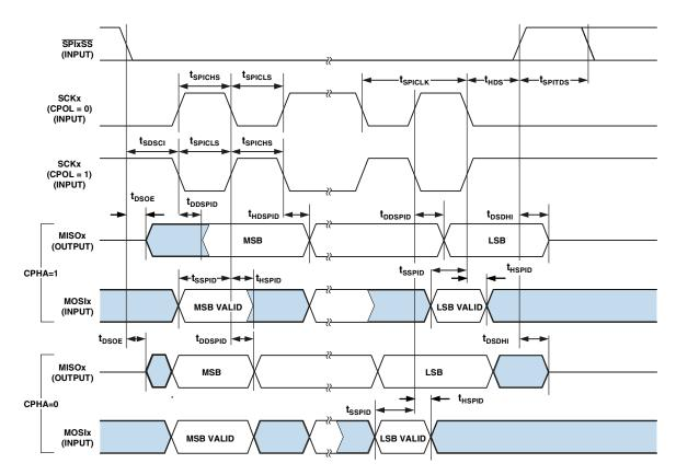
Figure 26. Serial Peripheral Interface (SPI) Ports—Slave Timing
