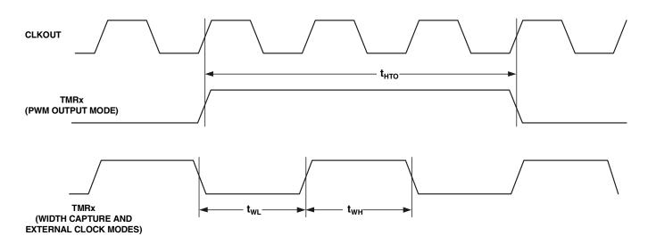
Figure 28. Timer PWM\_OUT Cycle Timing
