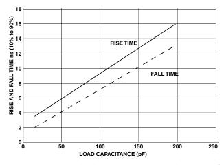
Figure 49. Typical Rise and Fall Times (10% to 90%) vs. Load Capacitance for Driver D at  $V_{DDEXT} = 2.7 V$  (MIN)
