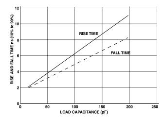
Figure 45. Typical Rise and Fall Times (10% to 90%) vs. Load Capacitance for Driver B at  $V_{DOEXT} = 2.7 V$  (MIN)
