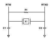
$\begin{array}{l} \text{SUGGESTED COMPONENTS:} \\ \text{ECLIPTEK EC38J (THROUGH-HOLE PACKAGE)} \\ \text{EPSON MC405 12 pF LOAD (SURFACE-MOUNT PACKAGE)} \\ \text{C1 = 22pF} \\ \text{C2 = 22pF} \\ \text{R1 = 10M\Omega} \\ \text{NOTE: C1 AND C2 ARE SPECIFIC TO CRYSTAL SPECIFIED FOR X1.} \\ \text{CONTACT CRYSTAL MANUFACTURER FOR DETAILS. C1 AND C2} \\ \text{SPECIFICATIONS ASSUME BOARD TRACE CAPACITANCE OF 3pF.} \end{array}$
