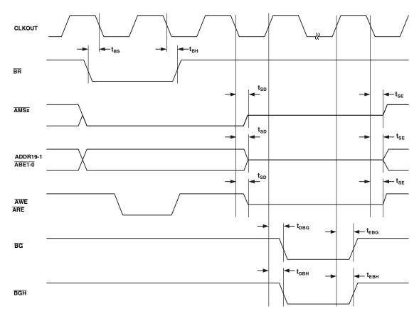
Figure 17. External Port Bus Request and Grant Cycle Timing with Synchronous BR
