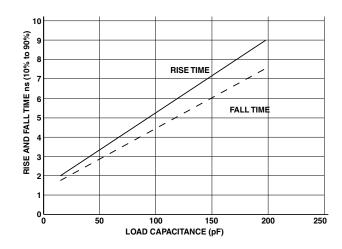
Figure 46. Typical Rise and Fall Times (10% to 90%) vs. Load Capacitance for Driver B at V<sub>DDEXT</sub> = 3.65 V (MAX)
