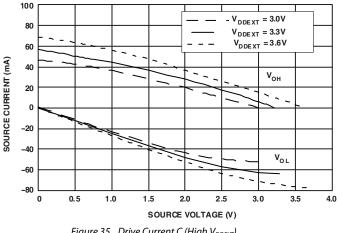
Figure 35. Drive Current C (High V<sub>DDEXT</sub>)
