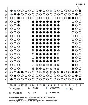
*Figure 54. 316-Ball CSP\_BGA Ball Assignment (Bottom View)*
