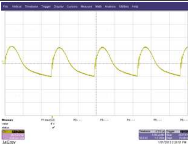
Figure 43. Ripple with 5-V, 1.2-A Output, 85 V AC Input, 20 mV/div, 5 \mu s/div
