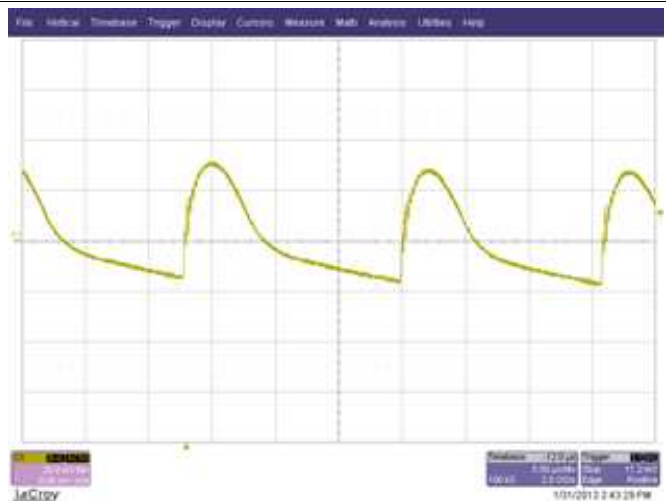
Figure 44. Ripple with 5-V, 1.2-A Output, 265-V AC Input, 20 mV/div 5 \mu s/div
