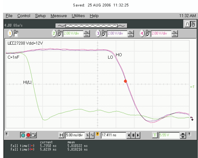
Figure 27. V_{LO} and V_{HO} Fall Time, 1-nF Load, 5-ns/Div
