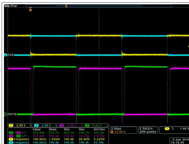
Figure 41. Bench Test Waveform for INA/B and OUTA/B
