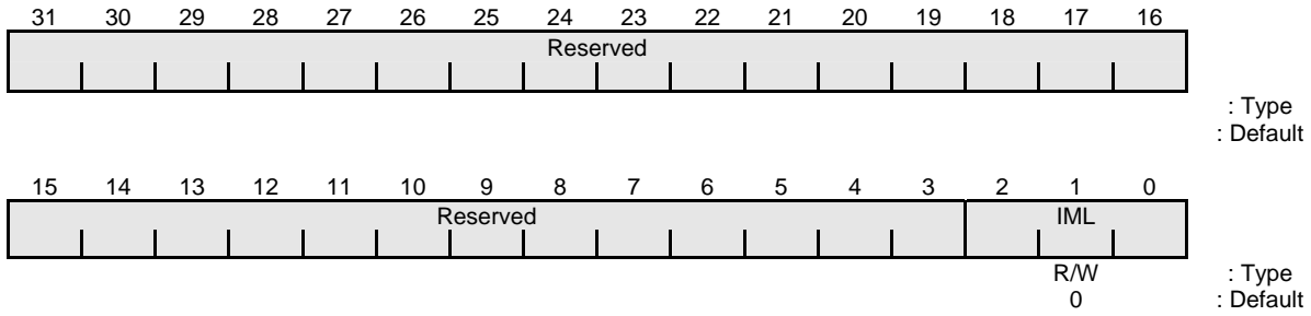
Figure 8-10 Interrupt Mask Level Register
