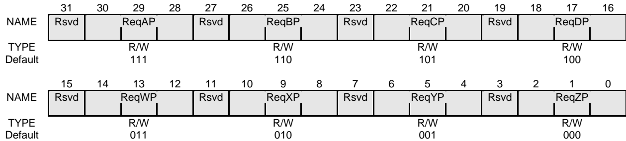
Figure 16-33 PCI Bus Arbiter Request Port Register
