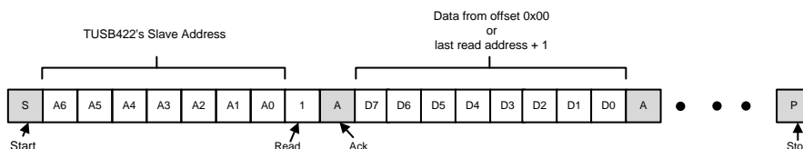
Figure 7. I2C Read Without Repeated Start
