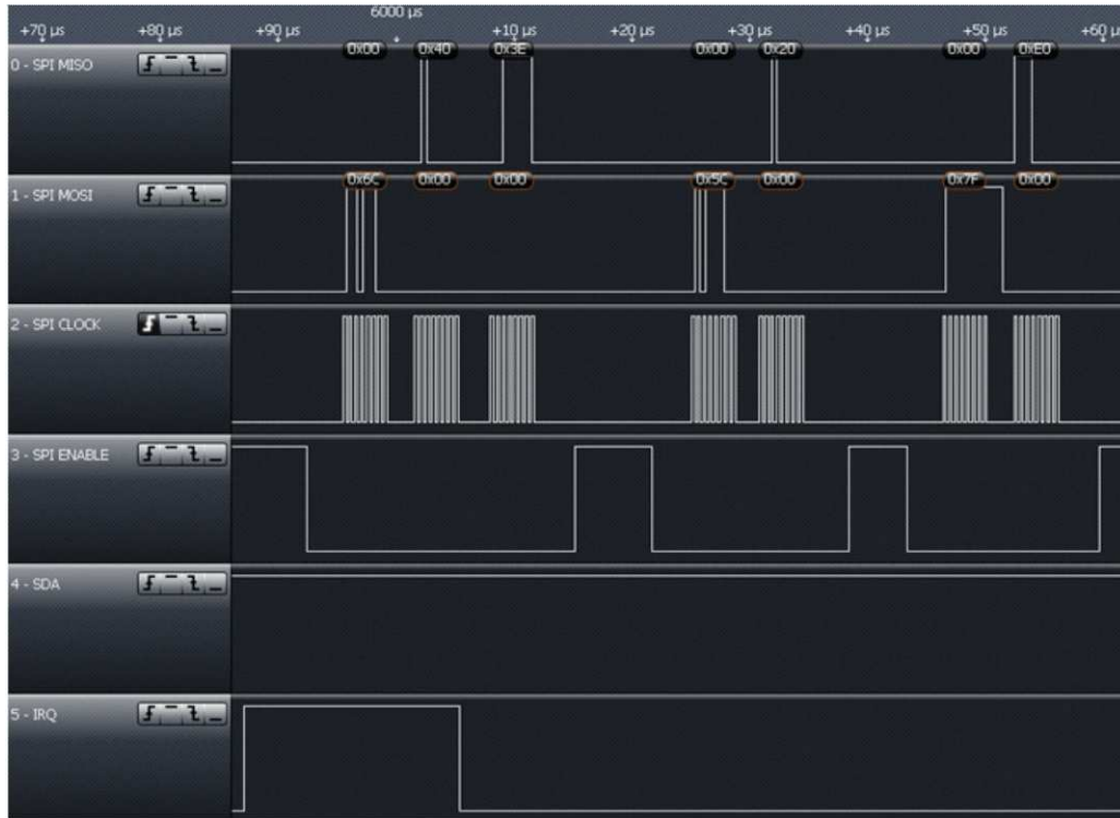
Figure 5-24. IRQ With One Byte in FIFO
