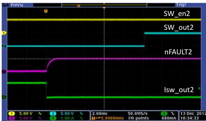
Figure 44. USB Switch2 Current Limit Recovery
