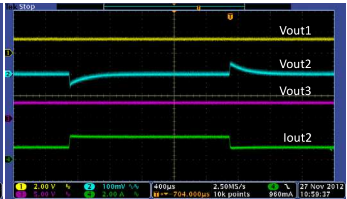
Figure 23. Transient Response Buck2@1.8V, 1-2A Step, C_o = 47\ \mu\text{F}
