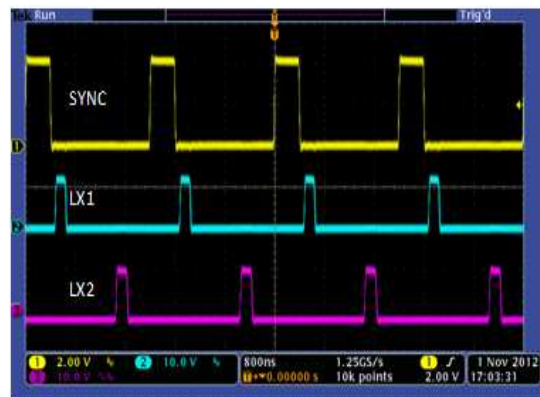
Figure 32. Synchronization at 500 kHz
