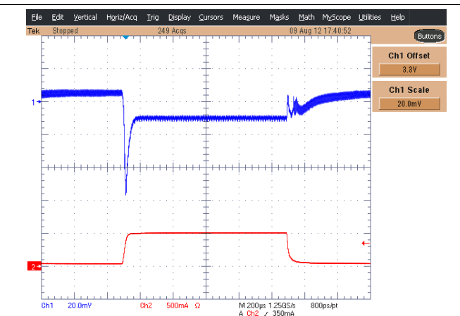
Figure 70. DCDC Load Transient, 3.3 V Out, 50-500-50
