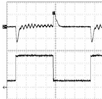
Figure 20. Overcompensated (Damped Oscillation), R_c Is Too Large
