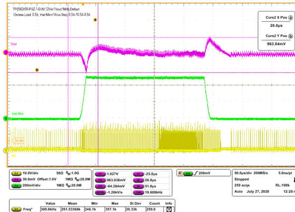
Figure 6-25. Overvoltage Protection, Negative OCP, then Undervoltage Protection by Load Stepdown
