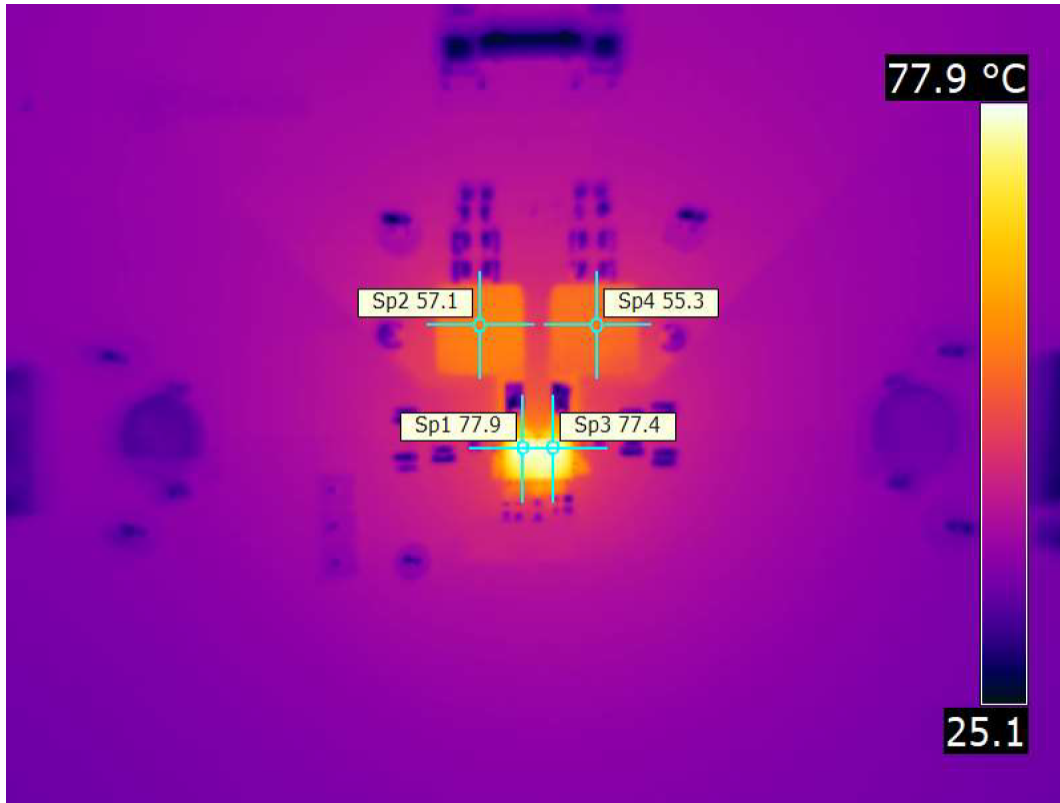
Figure 10-4. Thermal Image at 25°C Ambient - Dual Output Operation, f_{sw} = 1 \text{ MHz} , V_{IN} = 12 \text{ V} , V_{OUT1} = 1 \text{ V} , I_{OUT1} = 6 \text{ A} , L_1 = 560 \text{ nH} (3.3 mΩ Max), V_{OUT2} = 3.3 \text{ V} , I_{OUT2} = 6 \text{ A} , L_2 = 1.2 \text{ } \mu\text{H} (7.5 mΩ Max)
