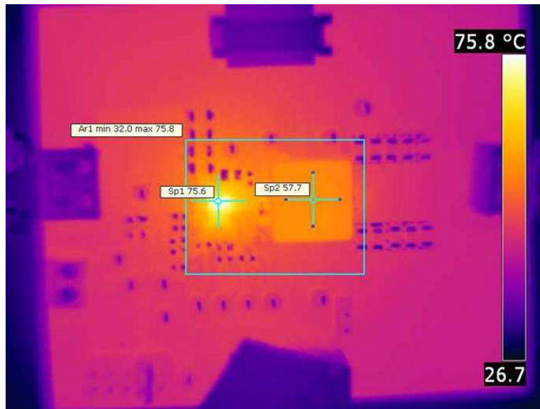
Figure 32. SP1: 75.6°C (TPS53515), SP2: 57.7 °C (Inductor)
