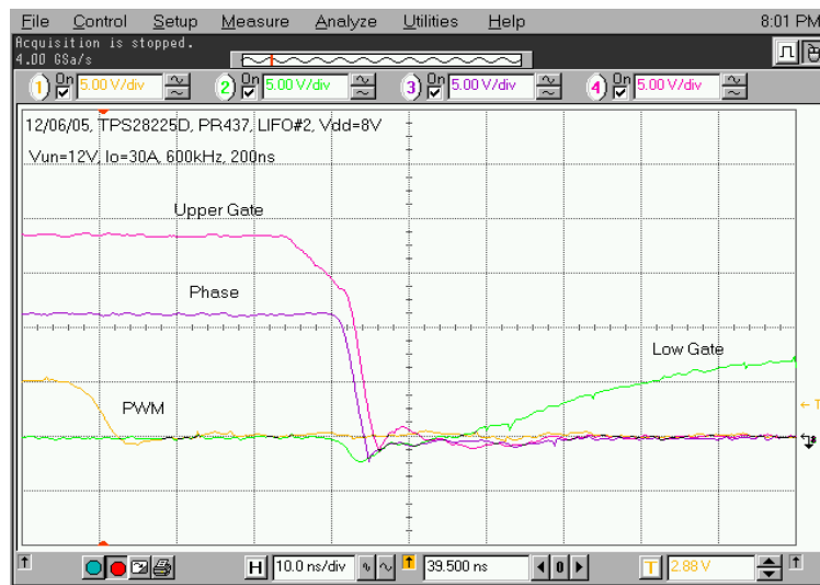
Figure 40. Phase Falling Edge Switching Waveforms (10 ns/div) of the Power State in Figure 31
