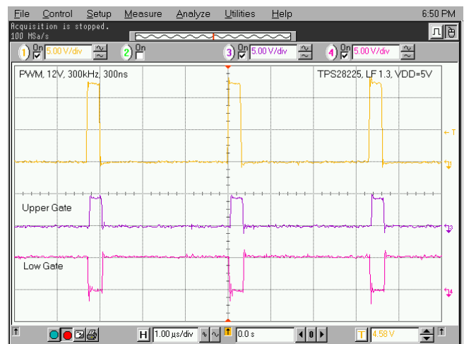
Figure 23. 12-V PWM Pulse at V_{DD} = 5 V
