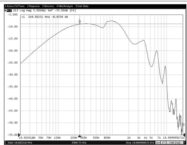
Figure 8-32. Off-State Data-Switch Isolation vs Frequency (TPS25832-Q1)
