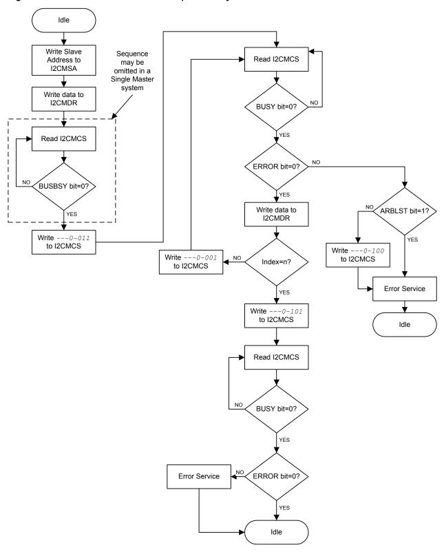
Figure 16-10. Master TRANSMIT of Multiple Data Bytes
