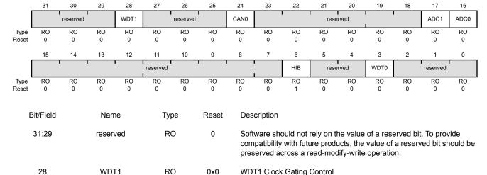
This bit controls the clock gating for the Watchdog Timer module 1. If set, the module receives a clock and functions. Otherwise, the module is unclocked and disabled. If the module is unclocked, a read or write to the module generates a bus fault.
