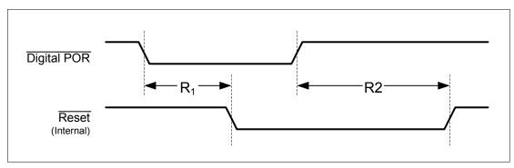
**Note:** The digital Power-On Reset is only released when the analog Power-On Reset has deasserted and all of the Power-OK monitors for each of the supplies indicate that power levels are in operational ranges.
