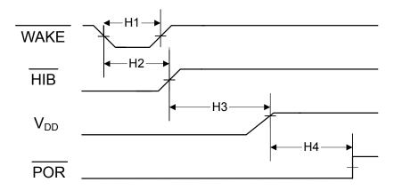
b. For recommended V<sub>BAT</sub> RC circuit values, refer to the diagrams located in "Hibernation Clock Source" on page 467.
