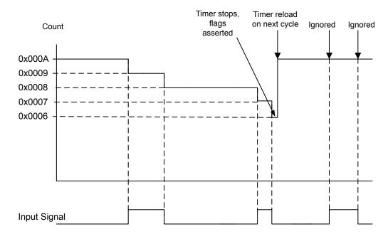
Figure 11-3. Input Edge-Count Mode Example, Counting Down
