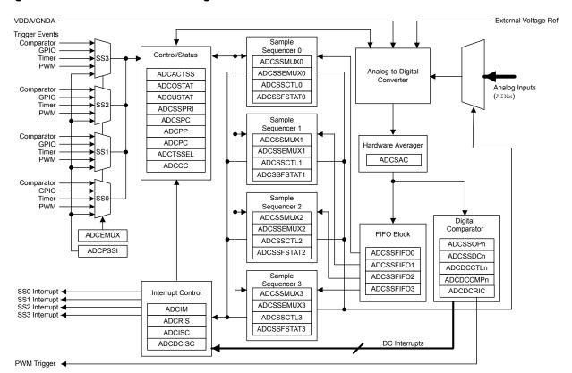
Figure 13-2. ADC Module Block Diagram
