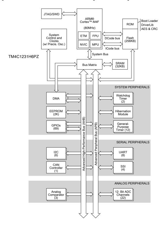
Figure 1-1. Tiva<sup>™</sup> TM4C1231H6PZ Microcontroller High-Level Block Diagram
