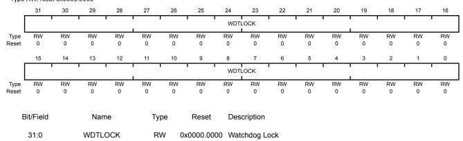
A write of the value 0x1ACC.E551 unlocks the watchdog registers for write access. A write of any other value reapplies the lock, preventing any register updates, except for the **WDTTEST** register. Avoid writes to the **WDTTEST** register when the watchdog registers are locked.
