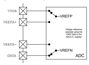
The range of this conversion value is from 0x000 to 0xFFF. In single-ended-input mode, the 0x000 value corresponds to the voltage level on VREFN; the 0xFFF value corresponds to the voltage level on VREFP. This configuration results in a resolution that can be calculated using the following equation:
