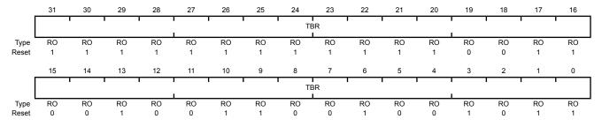
Bit/Field Name Type Reset Description 31:0 **TBR** RO
