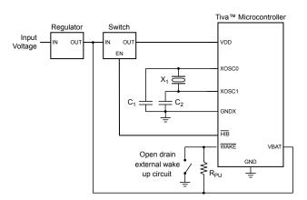
Figure 7-4. Using a Regulator for Both V<sub>DD</sub> and V<sub>BAT</sub>
