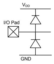
Table 21-31. Non-Fail-Safe I/O Pad Voltage/Current Characteristics abcd
