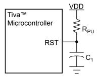
$R_{PU}$  = 1 k $\Omega$  to 100 k $\Omega$
