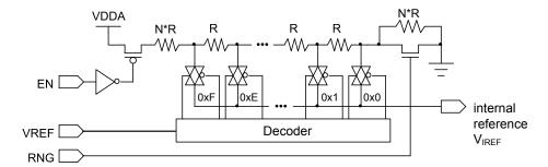
**Note:** In the figure above, N\*R represents a multiple of the R value that produces the results specified in Table 18-2 on page 1080.
