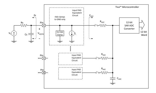
The ADC operates from both the 3.3-V analog and 1.2-V digital power supplies. The ADC clock can be configured to reduce power consumption when ADC conversions are not required (see "System Control" on page 215). The analog inputs are connected to the ADC through specially balanced input paths to minimize the distortion and cross-talk on the inputs. Detailed information on the ADC power supplies and analog inputs can be found in "Analog-to-Digital Converter (ADC)" on page 1155.
