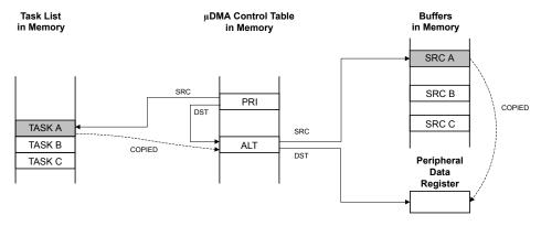
Using the channel's primary control structure, the  $\mu DMA$  controller copies task A configuration to the channel's alternate control structure.
