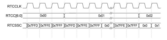
In the case of a trim value below 0x7FFF, the RTCSSC value is advanced from 0x7FFF to the trim value while the RTCC value is incremented from 0x0 to 0x1. If the match value is within that range, the match interrupt is not triggered. For example, as shown in Figure 7-6 on page 471, if the match interrupt was configured with RTCM0=0x1 and RTCSSM=0x2, an interrupt would never be triggered.
