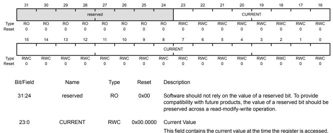
No read-modify-write protection is provided, so change with care. This register is write-clear. Writing to it with any value clears the register.
