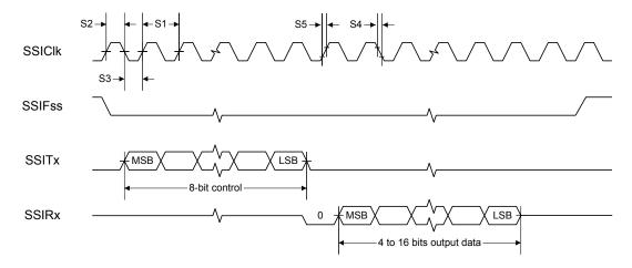
Figure 21-22. Master Mode SSI Timing for SPI Frame Format (FRF=00), with SPH=1
