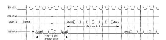
Figure 15-11. MICROWIRE Frame Format (Continuous Transfer)
