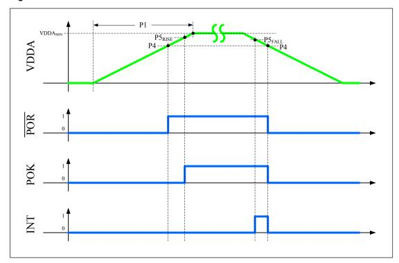
Figure 21-4. Power Assertions versus VDDA Levels
