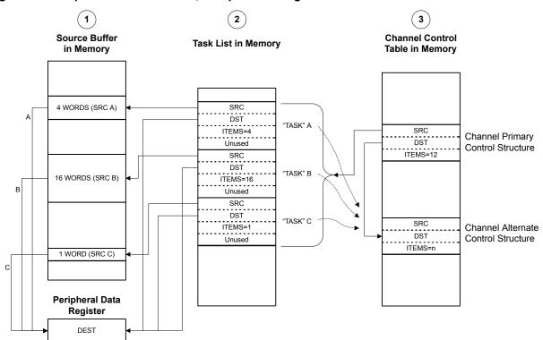
Figure 9-5. Peripheral Scatter-Gather, Setup and Configuration
