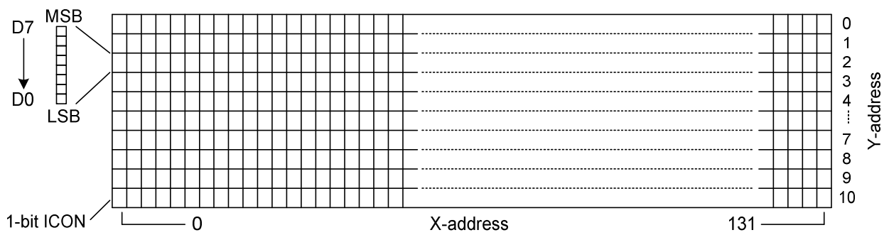
Figure 15 RAM format and addressing, if DO=1
