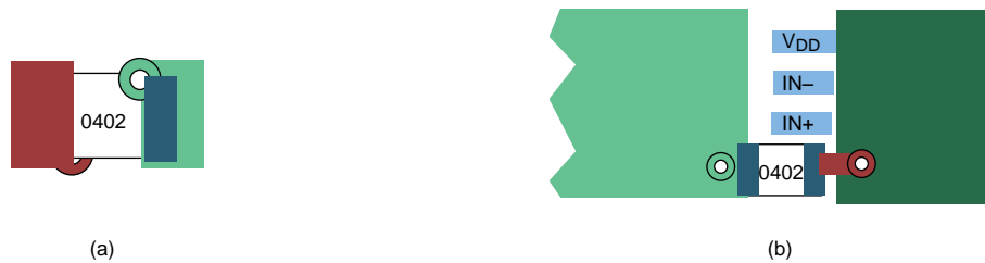
Figure 33. Typical Decoupling Capacitor Layouts
