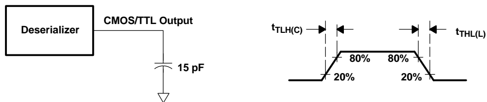
Figure 5. Deserializer CMOS/TTL Output Load and Transition Times
