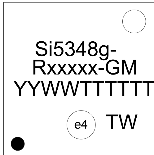
Figure 13.1. Si5348 Top Marking
