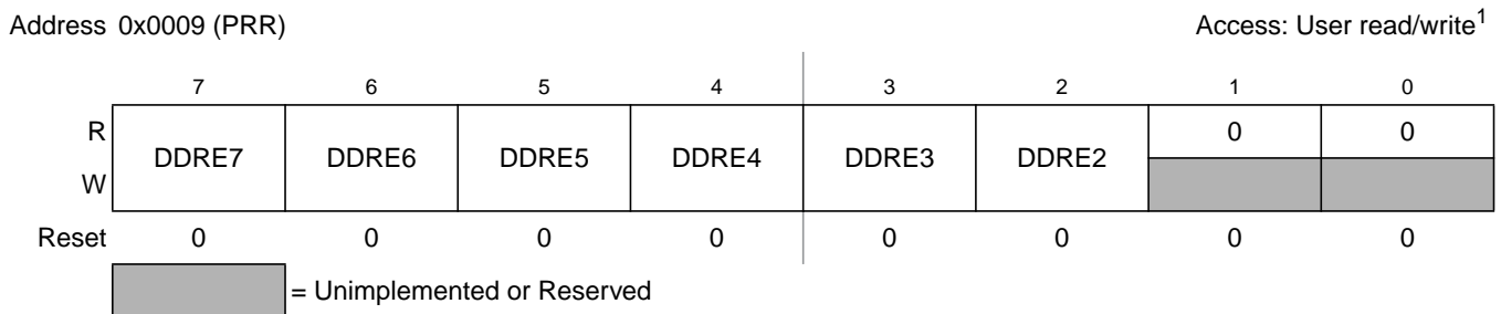
Figure 2-7. Port E Data Direction Register (DDRE)
