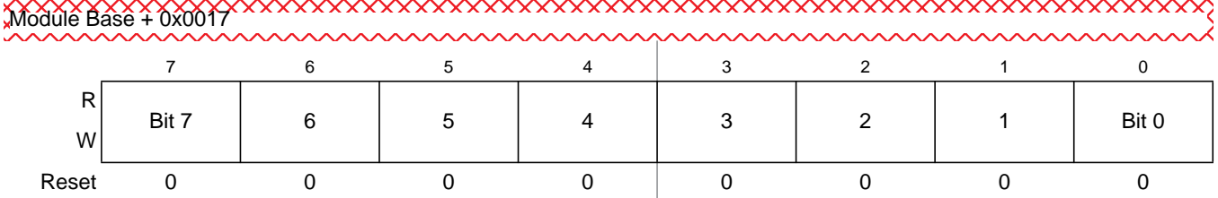
Figure 10-26. PWM Channel Period Registers (PWMPER5)
