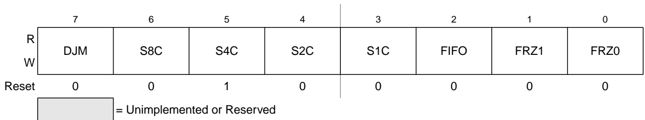
Figure 9-6. ATD Control Register 3 (ATDCTL3)
