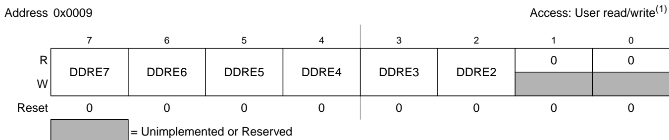
Figure 2-7. Port E Data Direction Register (DDRE)
