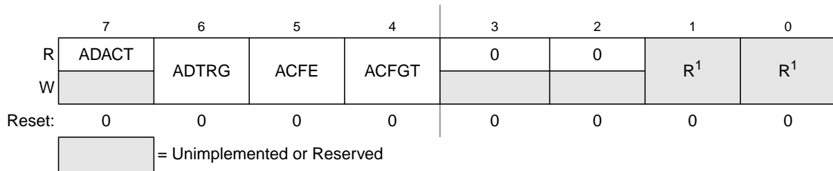
Figure 9-5. Status and Control Register 2 (ADCSC2)
