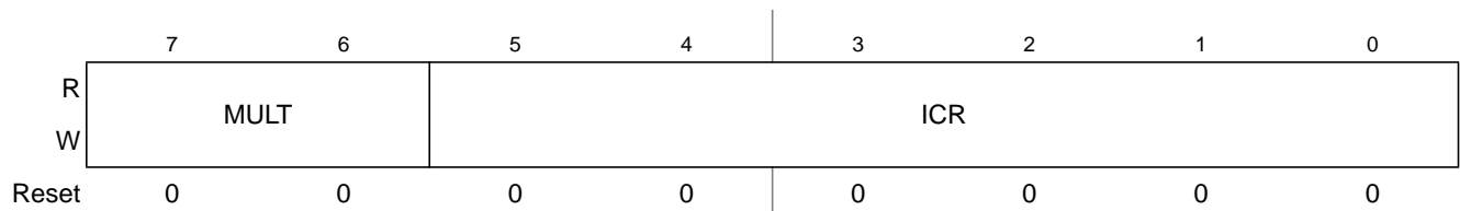
Figure 11-4. IIC Frequency Divider Register (IICF)
