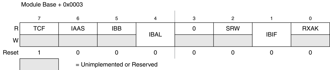
Figure 15-7. IIC Bus Status Register (IBSR)
