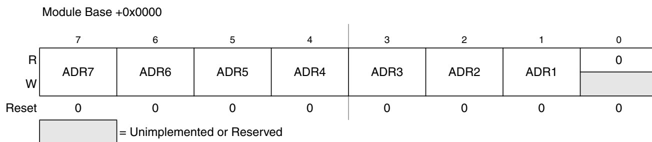
Figure 15-3. IIC Bus Address Register (IBAD)
