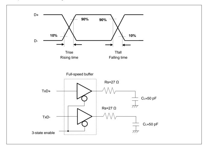
6. USB Full-speed connection is performed via twist pair cable shield with 90  $\Omega \pm 15\%$  characteristic impedance (Differential Mode).
