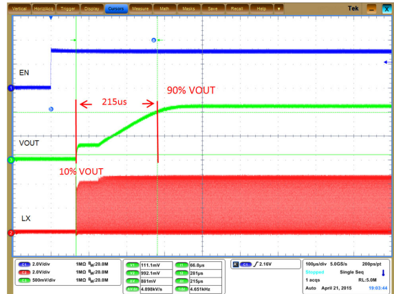
Figure 16. Soft-start Time for NCP6323D ( V_{IN} = 4.2\text{ V} , V_{OUT} = 1.1\text{ V} , I_{OUT} = 0\text{ A} , L = 1\text{ }\mu\text{H} , C_{OUT} = 10\text{ }\mu\text{F} )
