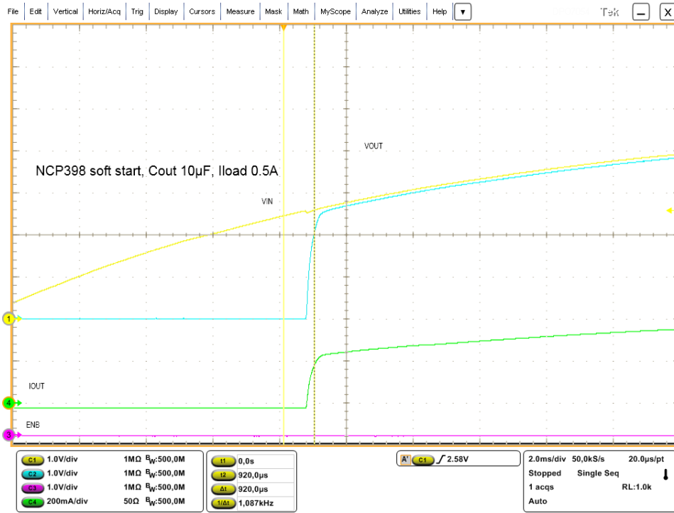
Figure 12. Soft Start On Cout 10 \mu F, 500 mA, Vin: yellow, Vout: blue, \overline{\text{EN}} : pink, IOUT: green
