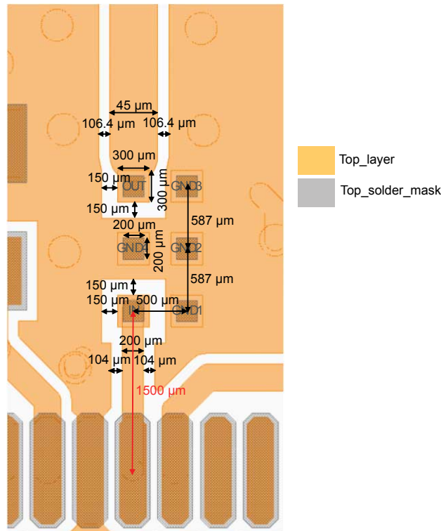
Figure 13. PCB land pattern recommendations
