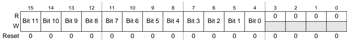
Figure 24-14. Left justified ATD conversion result register (ATDDR n )
