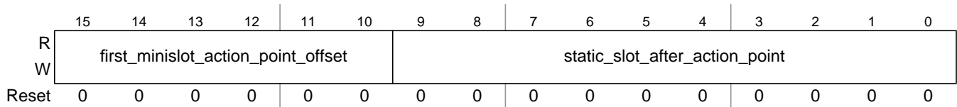
Figure 13-78. Protocol Configuration Register 13 (PCR13)
