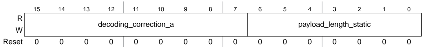
Figure 13-84. Protocol Configuration Register 19 (PCR19)
