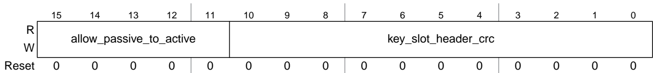
Figure 13-77. Protocol Configuration Register 12 (PCR12)
