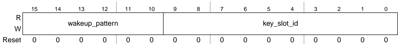
Figure 13-83. Protocol Configuration Register 18 (PCR18)
