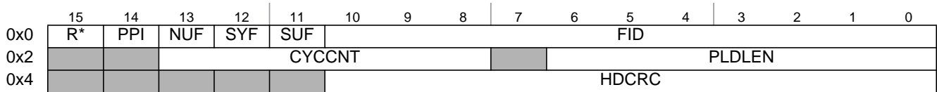
Figure 13-105. Frame Header Structure
