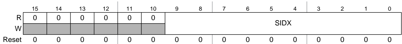
Figure 13-53. Receive FIFO Start Index Register (RFSIR)
