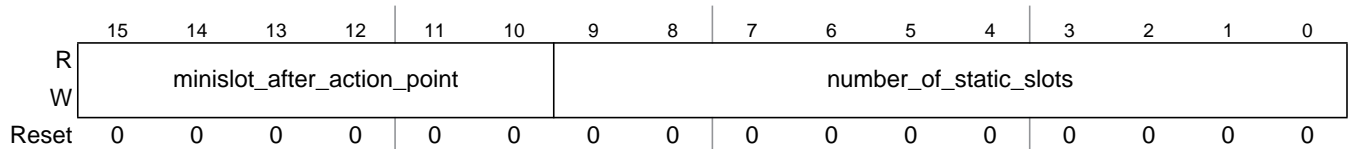
Figure 13-67. Protocol Configuration Register 2 (PCR2)
