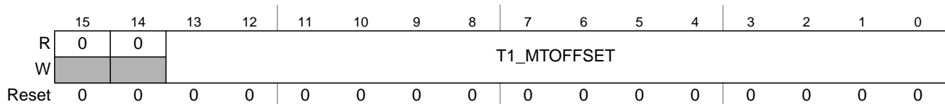
Figure 13-42. Timer 1 Macrotick Offset Register (T1MTOR)
