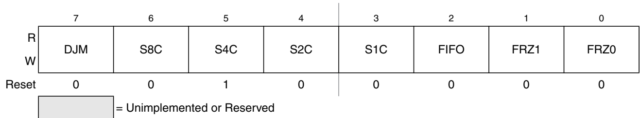
Figure 13-6. ATD Control Register 3 (ATDCTL3)
