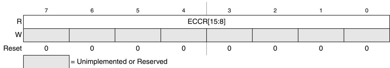
Figure 28-20. Flash ECC Error Results High Register (FECCRHI)
