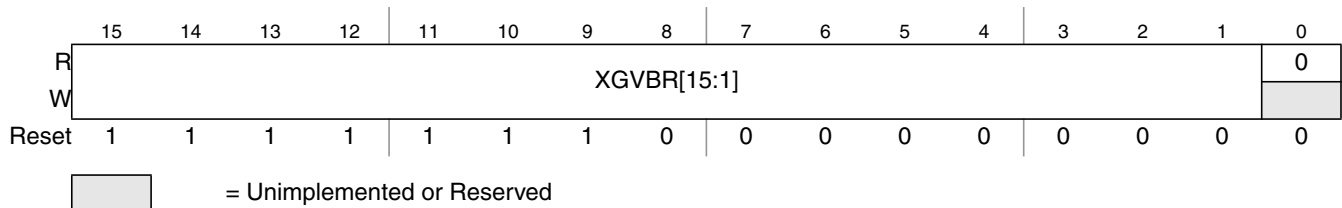
Figure 10-9. XGATE Vector Base Address Register (XGVBR)
