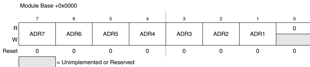
Figure 15-3. IIC Bus Address Register (IBAD)
