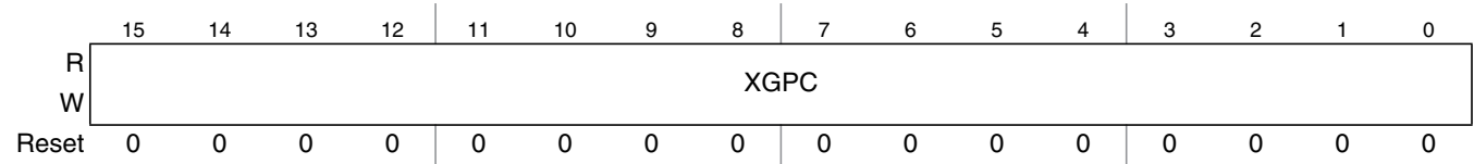
Figure 10-14. XGATE Program Counter Register (XGPC)
