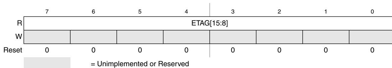
Figure 28-18. EEE Tag Counter High Register (ETAGHI)
