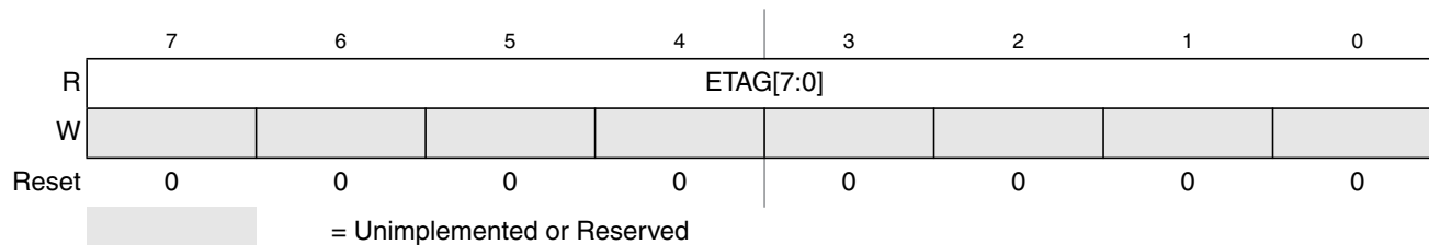
Figure 28-19. EEE Tag Counter Low Register (ETAGLO)
