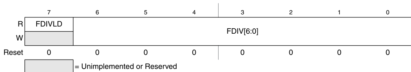
Figure 25-5. Flash Clock Divider Register (FCLKDIV)
