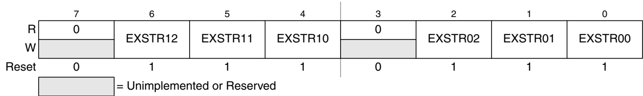
Figure 5-4. External Bus Interface Control Register 1 (EBICTL1)
