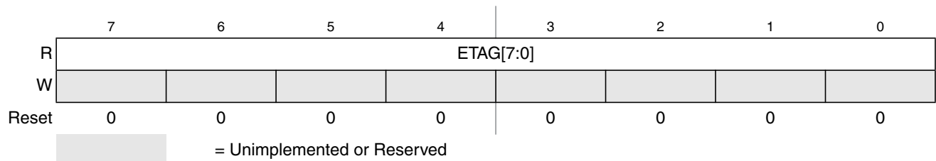
Figure 25-19. EEE Tag Counter Low Register (ETAGLO)
