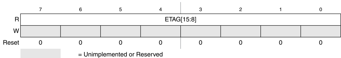
Figure 24-18. EEE Tag Counter High Register (ETAGHI)
