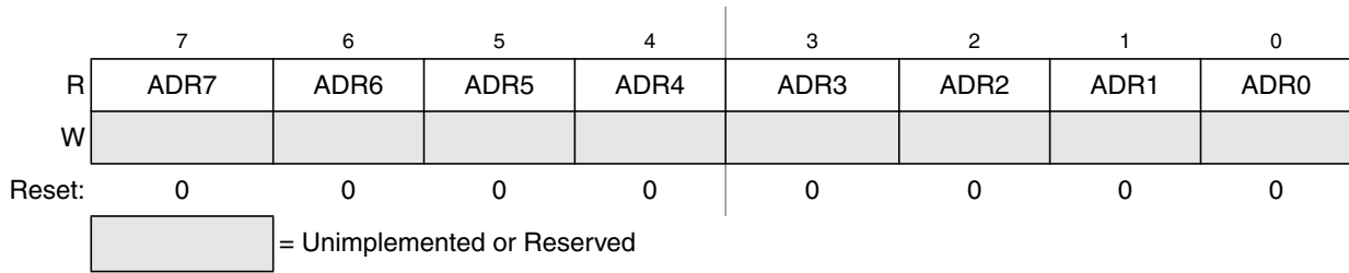
Figure 14-7. Data Result Low Register (ADC1RL)
