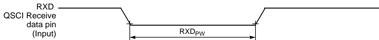
Figure 10-12 RXD Pulse Width
