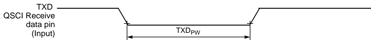
Figure 10-13 TXD Pulse Width
