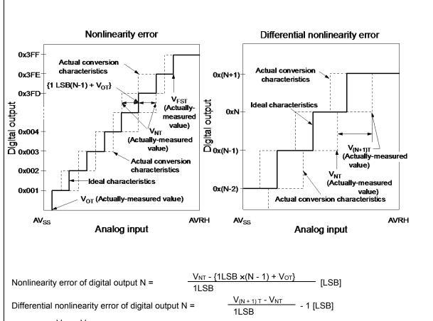
$1LSB = \frac{V_{FST} - V_{OT}}{1022}$
