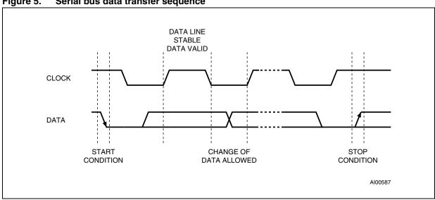
Figure 5. Serial bus data transfer sequence
