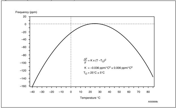
Figure 13. Clock calibration
