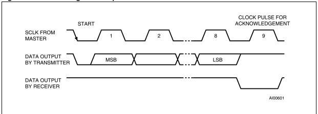
Figure 7. Bus timing requirements sequence
