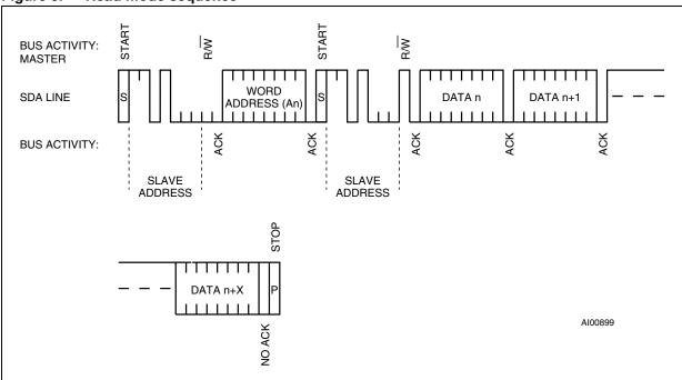
Figure 10. Alternate read mode sequence
