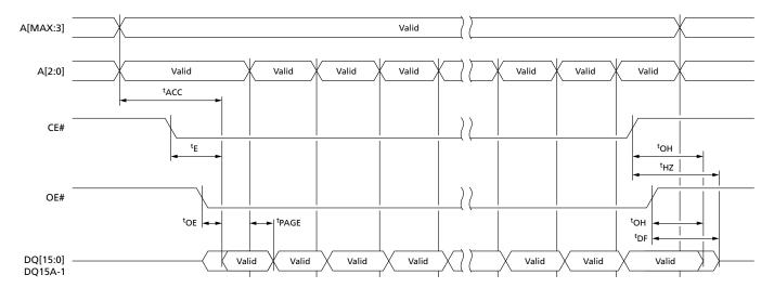
Note: 1. Page size is 8 words (16 bytes) and is addressed by address inputs A[2:0] in x16 bus mode and A[2:0] plus DQ15/A-1 in x8 bus mode.
