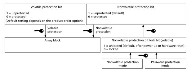
Notes: 1. Volatile protection bits are programmed and cleared individually. Nonvolatile protection bits are programmed individually and cleared collectively.
