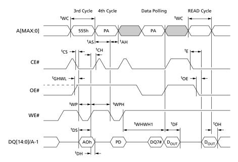
Only the third and fourth cycles of the PROGRAM command are represented. The PRO-GRAM command is followed by checking of the status register data polling bit and by a READ operation that outputs the data (D<sub>OUT</sub>) programmed by the previous PROGRAM command.
