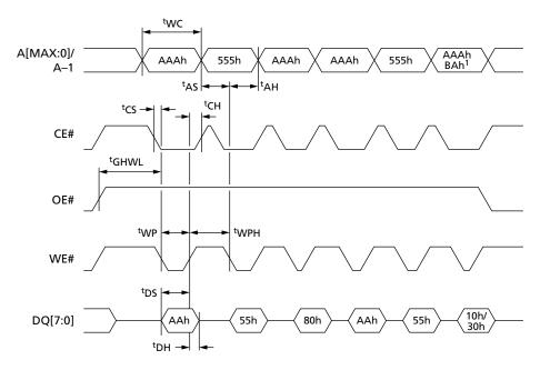
Notes: 1. For a CHIP ERASE command, the address is AAAh, and the data is 10h; for a BLOCK ERASE command, the address is BAd, and the data is 30h.
