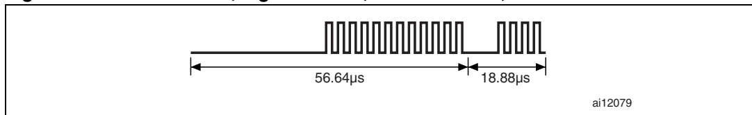
Figure 36. Start of frame, high data rate, one subcarrier, fast commands
